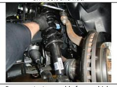
Remove strut assembly from vehicle
