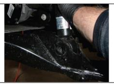
Push down suspension and reinstall lower strut bolt and nut.
