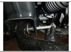
Torque lower control arm hardware at ride height. Lift lower control arm into position and reinstall bolts.
