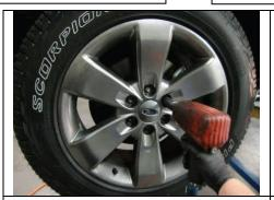
Raise and support front of vehicle off the ground. Remove front wheels/tires, support suspension with jack.
