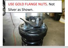
Install new strut extension with GOLD Flange Nuts, tighten.
