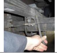
Remove u-bolts and carefully lower axle.
