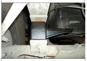
Remove factory block and replace with new, taller block.
