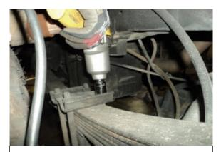
Remove U-bolt nuts on top of spring pack.
