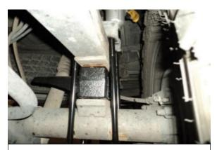
Raise the axle and secure with new, longer U-bolts and hardware.
