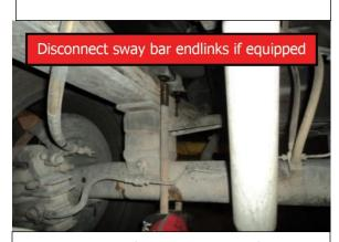
Remove U-bolts from axle and carefully lower the axle.
