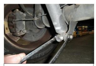
Remove the lower shock mount hardware.
