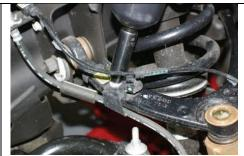
Disconnect ABS/brake bracket from upper control arm.
