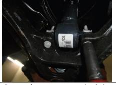
Remove lower strut mounting bolts
