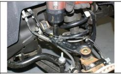
Reattach ABS/brake line bracket and sway bar end links
