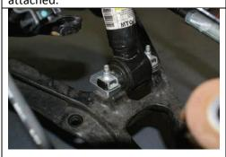
Image: Spacer installed
