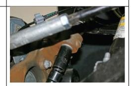
Tighten upper ball joint to spec.
