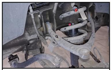
Disconnect the ABS connector at the frame rail; remove from UCA clip; remove the brake line bracket from UCA. Let hang out of the way. Remove the upper and lower strut hardware. Lower the strut out of the frame.
