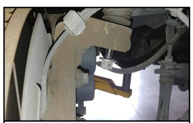
Loosen the upper ball joint nut. Strike the upper ball joint boss with a hammer to dislodge the taper. Remove the upper control arm from the knuckle. Lower the control arm with the jack to gain clearance to install the lower spacer.
