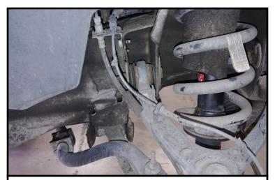
Install the brake line bracket to the upper control arm. Install the ABS wire to the bracket and frame rail. Reconnect the electrical connector. Install the sway bar to the frame rail. Install the wheels and tires. Have the alignment set.
