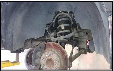
Support the lower control arm with a suitable jack. Remove the front wheels.
