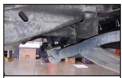
Remove the sway bar from the frame rail and let hang out of the way.
