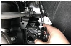
Remove ABS Bracket from UCA; Remove the brake line bracket from Knuckle.
