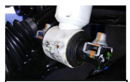
Remove factory clip nuts and discard. Supplied hardware will be used in its place. Install the lower strut spacer using the provided hardware.
