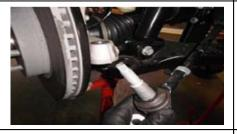
Remove the tie rod ends from the steering knuckle using a 21mm socket. Note: You may need to use a hammer to separate the ball joint from the knuckle.
