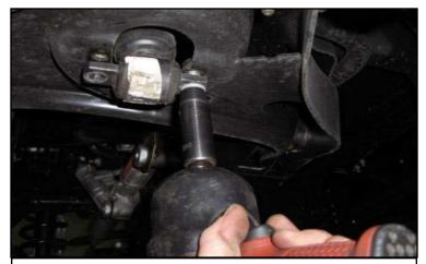
Support the lower control arm at the knuckle. Remove the lower shock hardware.
