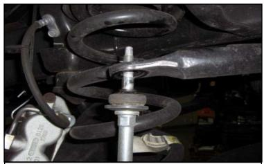
Raise vehicle. Remove front wheels. Remove the sway bar end links from the sway bar. Push sway bar up and out of the way.
