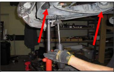
Remove the shock. Place jack stands at the pivot points of the lower control arm. Remove the lower control arm bolts at the frame.
