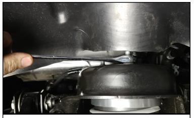
Remove the strut hardware at the lower control arm. Remove the upper strut hardware. Remove the strut from the vehicle.
