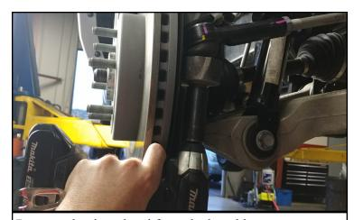
Remove the tie rod end from the knuckle.
