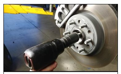
Remove the axle nut from the hub.
