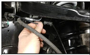
Remove the front wheels. Remove the ABS wire on the upper control arm, frame, and rubber brake line. Remove the metal brake line bracket at the frame.
