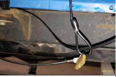
Short cable only hooks to one side of vehicle around body mount. Lock junction placed away from painted body to avoid damage.
