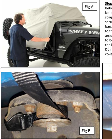
**Step 2:** Locate the side straps and attach below the door. Tighten straps slightly to keep them hooked on the vehicle. Once all straps are in place, tighten down evenly to secure the cover to the vehicle. Some nerf bars may prohibit the strap to be attached to the pinch weld. You may loop strap around body mount bolt and then attach to body mount cup or other location on the body tub. Fig B+C. Pull straps sung, but Do not over tighten straps, damage to cover and/or vehicle may occur.
