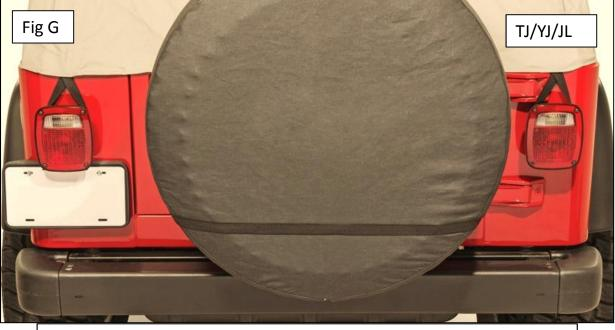
Center strap can go around the tire as shown or it can go around the tire carrier.
