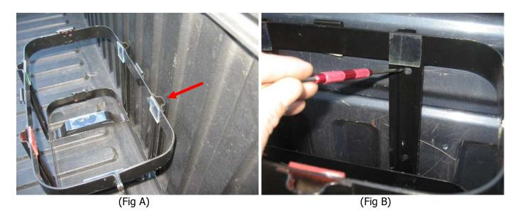
**Step 3:** Depending on the type of hardware you plan to use (Self Tapping bolts, Bolts with Nuts, ect) set the bracket to the side and drill the proper size mounting holes needed. You can purchase hardware at any home improvement store.
