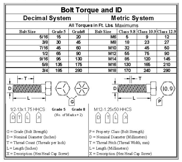
**NOTE:** Ford recommended maximum torque for 2021+ Bronco, OE 10mm threaded frame mounting holes is 50nm (36.8ft-lbs)
