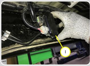
Once fuel pump module hardware is removed (*l*), hang module with a bungee cord or zip tie to support it. **DO NOT** let it hang from the wires.
