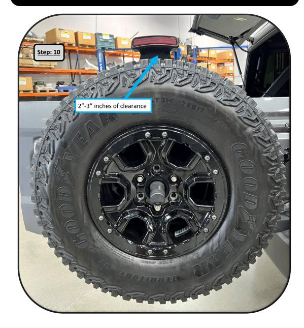
**Step 10:** Reinstall the spare tire and torque the OE lug nuts to 41ft-lbs. Reconnect the battery, install is complete.
