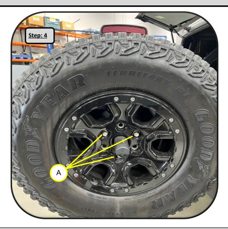
**Step 4:** Remove the (3qty) lug nuts **(Fig A.)** securing the Spare Tire to the tire carrier. Remove the Spare Tire and set aside.
