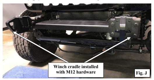
Step 12: Install the lower support gussets under the winch cradle to the back of the inside frame horn bolts, (Fig K) secure with M12 washers and lock nuts. Secure the winch cradle to the nut-plates installed in the frame supports (Step 10) with provided M12 bolts and washers through the support gussets.
