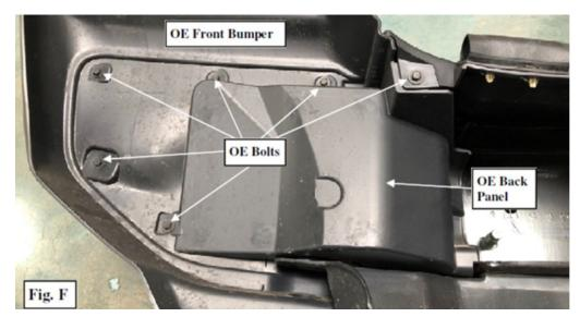
Step 8: Remove the (1 Per Side) OE plastic push rivet. Using a 7mm socket, remove the (1 Per Side) remaining OE screw securing the OE back panels to the OE front bumper. Remove the OE back panel from the OE front bumper. (Fig. G)
