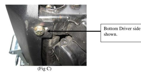
**STEP 3:** Make sure all bolts are securely tightened. Installation is now complete.
