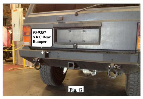
**Step 9:** Level the bumper and torque all mounting hardware according to the chart on page 15 or manufacturers specifications.
