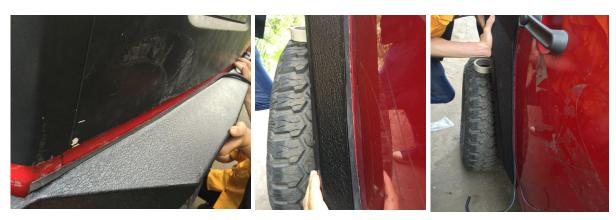
It is recommended to do a "dry" fitment first using clamps before proceeding with drilling an d a full install.
