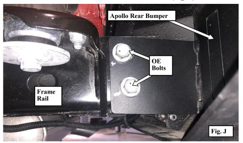
Step 17: Secure the Apollo rear bumper (77784) to the rear frame crossmember. Using (4)
