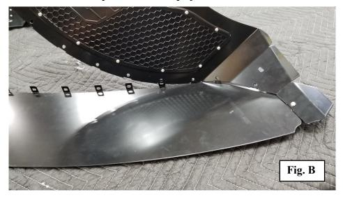
Step 3: With the front DS TOP PANEL now loosely attached to the DS BACK PANEL, slowly bend the TOP PANEL aligning the TOP PANEL mounting tabs, into the guide slots located along the top outer edge of the BACK PANEL. As you line up the hole for each tab, install the M6 hardware and hand-tighten (Fig. C).
