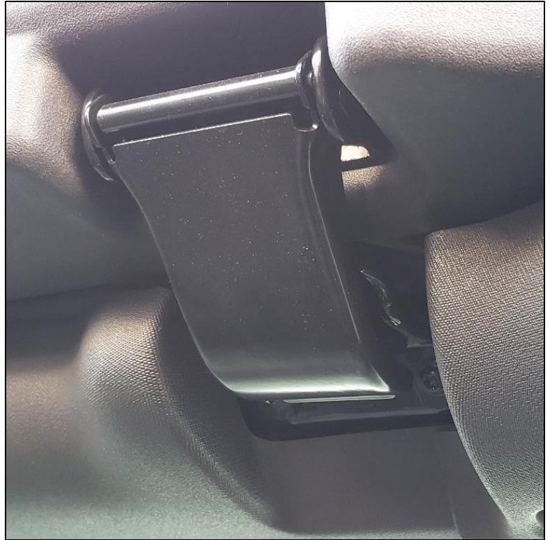
Windshield clamp in closed position.
