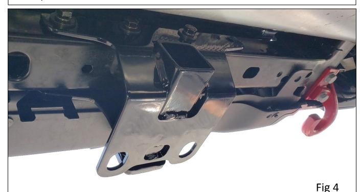
**Step 5:** Reinstall the M10 bolts from step 2 that secured the bottom of the bumper to the rear cross member, torque to 45 ft/lb. Then torque the nuts/bolts from step 1 to 45 ft/lb.
