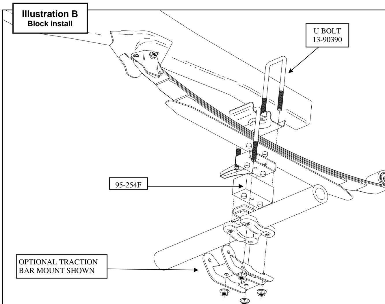
7. Support the rear axle with a floor jack and remove the **U-bolts** on the driver side. Loosen the **U-bolts** on the passenger side.
