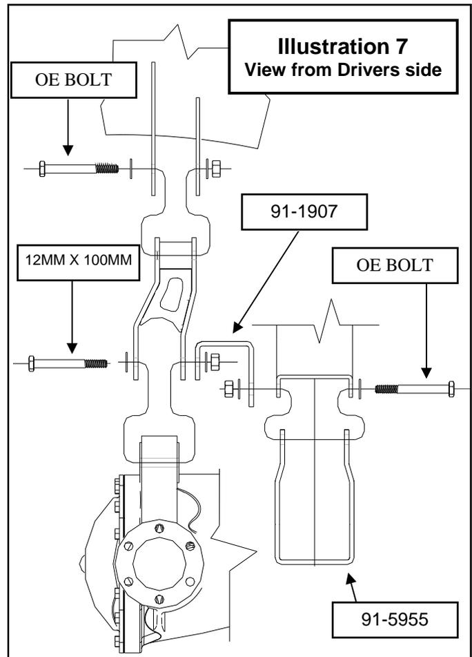
arms, do not tighten until the truck is on the ground.
