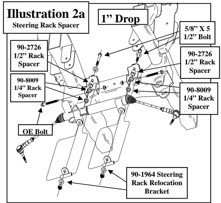
27. After installing the spacers to achieve a 1" drop, inspect for steering shaft and steering U-joint clearance at the frame.
