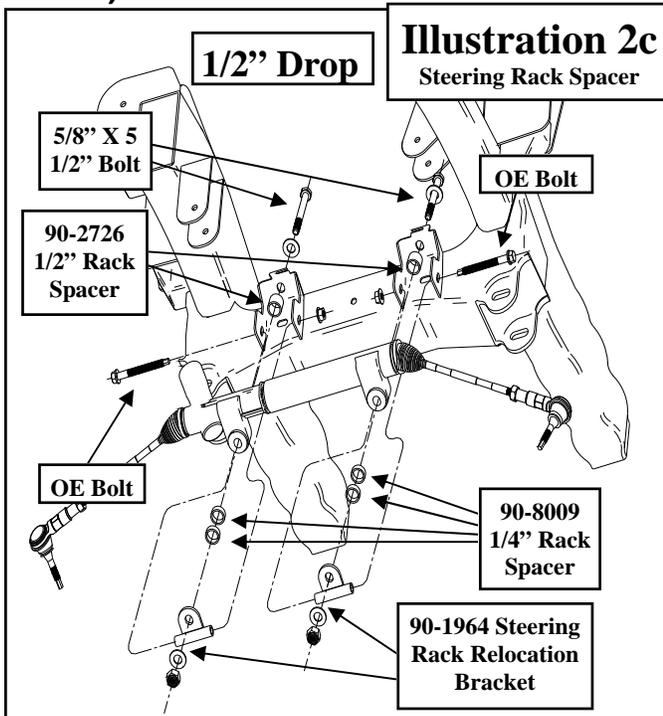
32. Check for steering shaft clearance to frame and band clamps, the dust boots and the clamps may have to be repositioned or removed. Torque the
