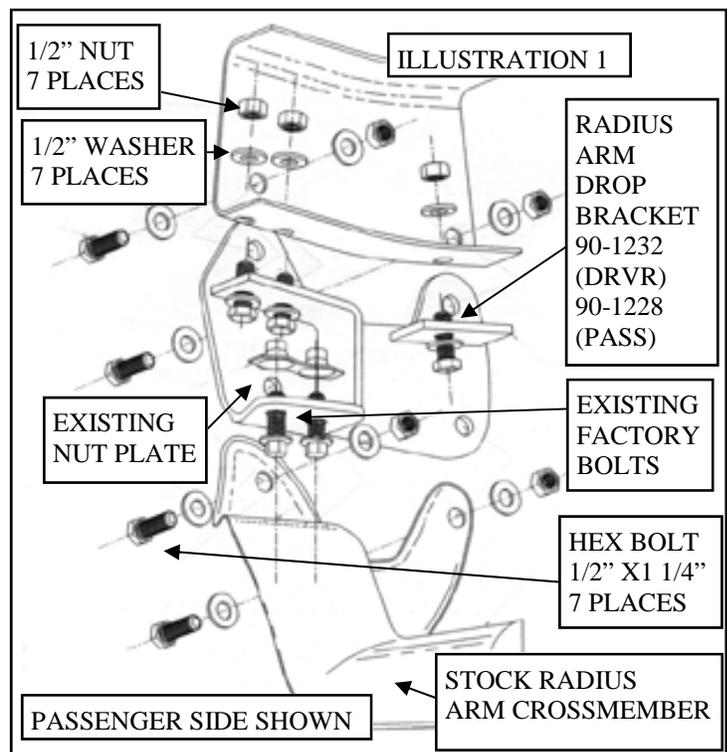
3) Loosen the bolts that attach the anti-sway bar to the radius arm brackets, if so equipped. Place a jack under the center of the crossmember. Raise jack until it touches the crossmember, but do not put a load on it. Remove the rivets and bolts that attach the radius arm brackets to the frame. See ILLUSTRATION 1. If a torch is used to remove the rivets, be careful not to damage the brackets, rubber body mounts, wiring or hoses located inside the frame.
