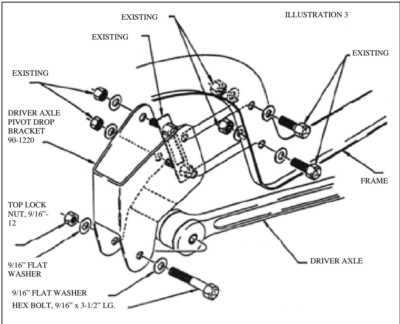
pivot hole as shown in ILLUSTRATION 2. Use the supplied 7/16" x 1-1/4" bolts and 7/16" washers and nuts in the remaining 3 holes. Apply loctite and tighten bolts. Attach passenger axle to axle pivot drop bracket using supplied 9/16" x 3-1/2" bolt and 9/16" washer and nut.
