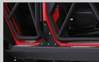
D B-pillar fixing point to reduce swaying
