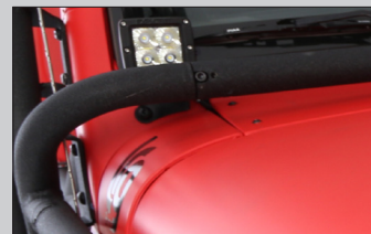
B 1.75" diameter 0.120-wall steel tubing
