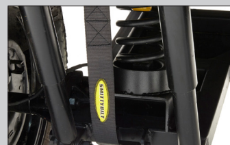
D Independent trailing arms, dual shocks and limiting straps
