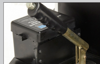
B Parking brake and electric break away system
