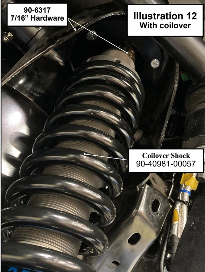
54. **IMPORTANT!** Rotate coil spring on the OE driver strut 180 degrees by using a spring compressor. Failure to do so will result in contact between coil and knuckle.
