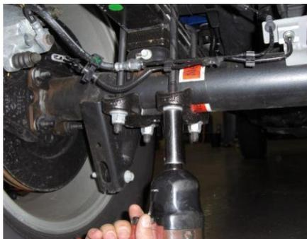
Loosen and remove factory u-bolt hardware.
