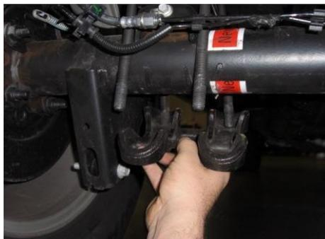
Remove u-bolt nuts and lower plate.
