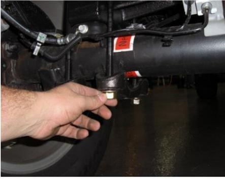
Attach lower mounting plate with provided hardware.
