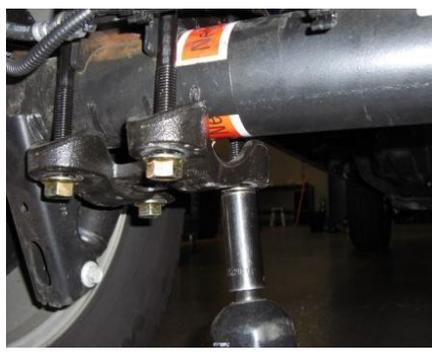
Snug hardware down, lower vehicle on ground and torque.
