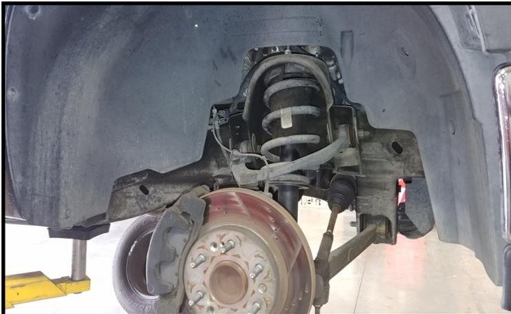
Support the lower control arm with a suitable jack. Remove the front wheels.
