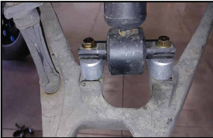
Install the lower strut spacer using the provided hardware. Raise the lower control arm up with the jack. You will have to load the suspension to install the upper control arm to the knuckle. Install the upper ball joint nut.
