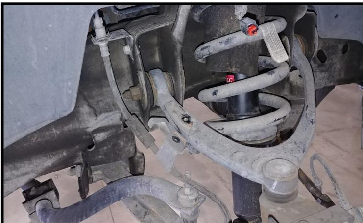
Disconnect the ABS connector at the frame rail; remove from UCA clip; remove the brake line bracket from UCA. Let hang out of the way. Remove the upper and lower strut hardware. Lower the strut out of the frame.
