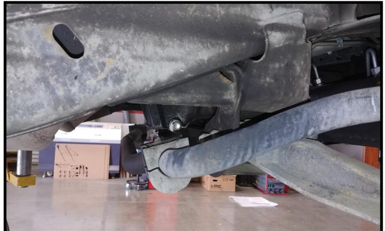
Remove the sway bar from the frame rail and let hang out of the way.
