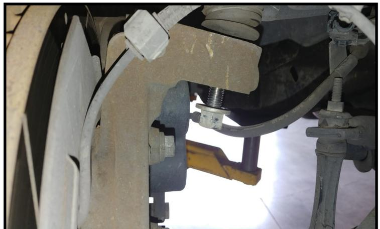
Loosen the upper ball joint nut. Strike the upper ball joint boss with a hammer to dislodge the taper. Remove the upper control arm from the knuckle. Lower the control arm with the jack to gain clearance to install the lower spacer.
