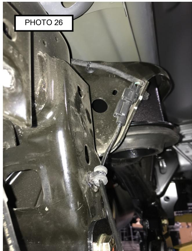
27. On both sides of the vehicle, check the routing of the brake lines and the ABS wire harnesses. There must be no pinching, rubbing, or stretching of either component. If necessary use zip ties to secure these lines out of the way and to keep from contacting any moving parts. Reposition them if needed.
