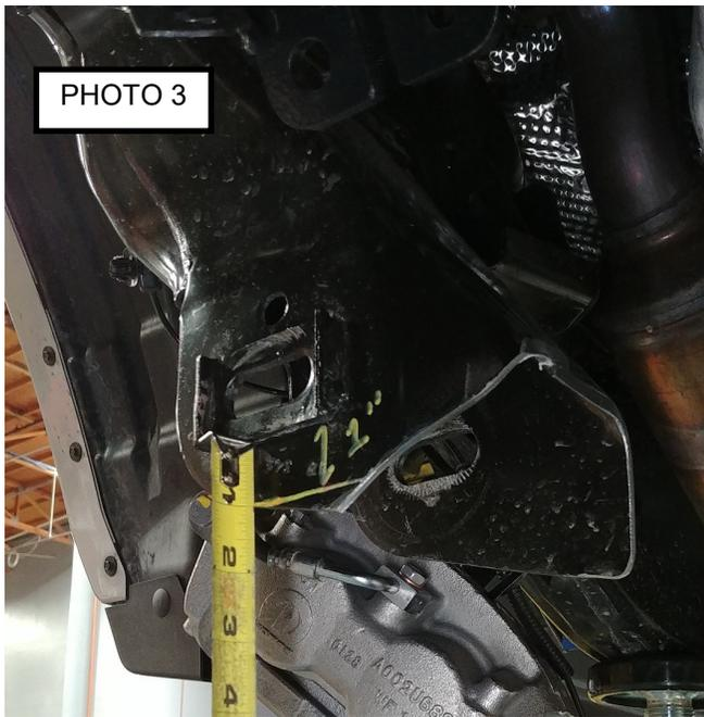
(2) M12 X 50mm flanged bolts and hardware from hardware pack (90-60728). Leave bolts loose at this time. **IMPORTANT!** The notch on the rib of the bracket will point towards the rear of the vehicle.
