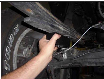
Place new lift block into position between axle and leaf pack.
