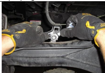
Replace shock on mount and ABS line to axle. Repeat steps on opposite side and torque when completed.
