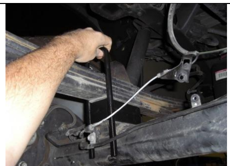
Slide new u-bolts over leaf pack and bump stop bracket.
