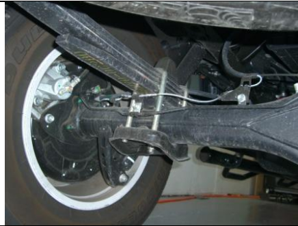
Work on one side at a time to prevent driveline damage.
