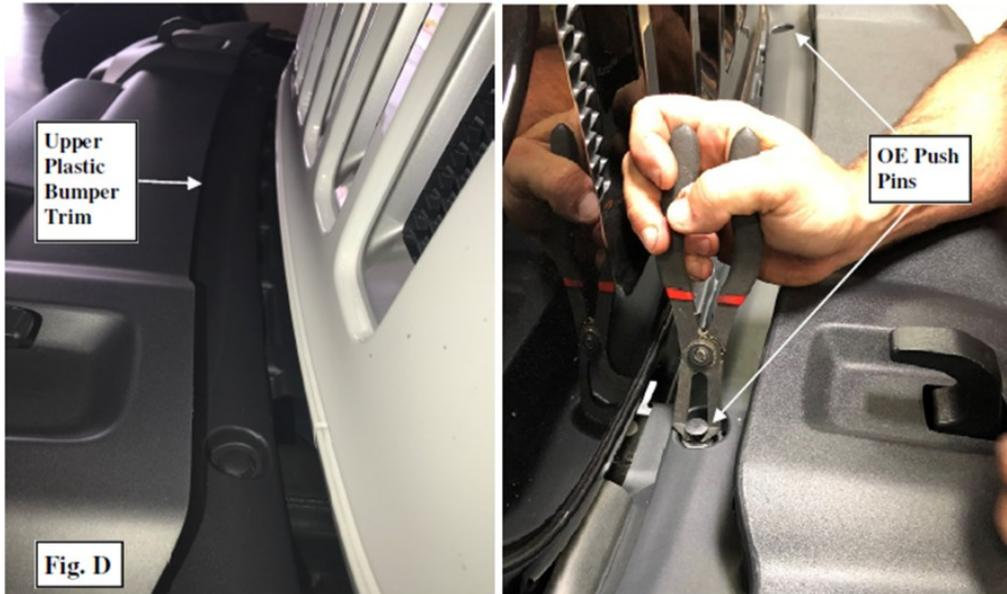
**Step 5** : Carefully remove the OE front bumper from the vehicle.
