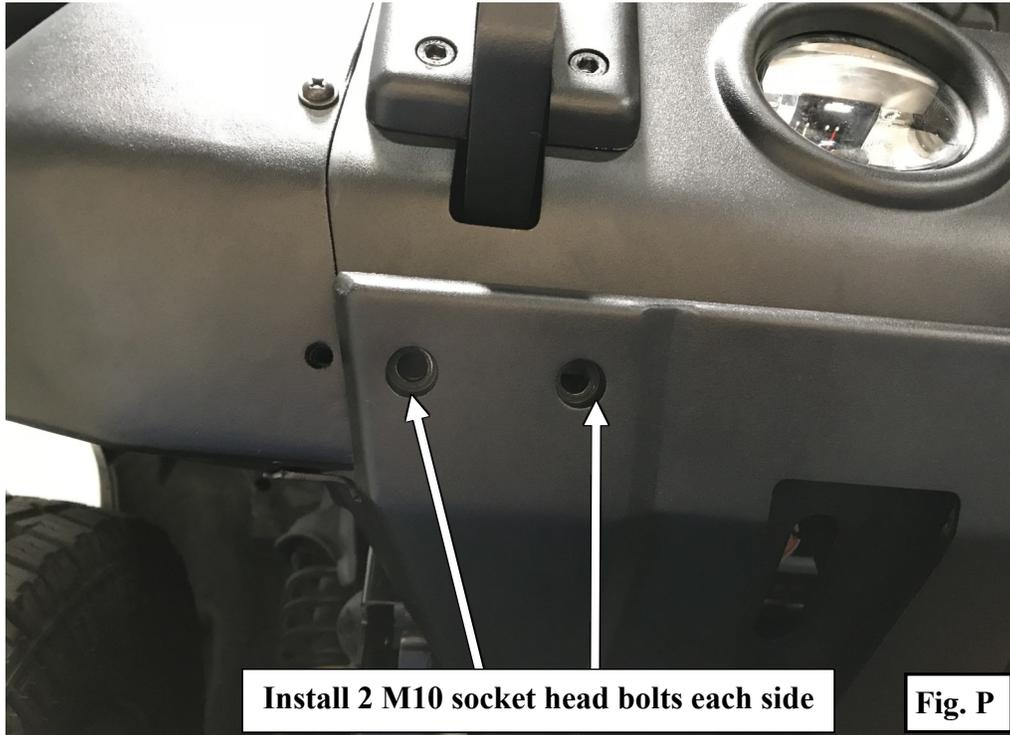
**Step 20:** If you have a JL go to Step 21. On JKs, bolt the lower portion of the skid plate to the crossmember Using supplied **M10 hardware**, tighten upper and lower hardware to 40ft-lbs.
